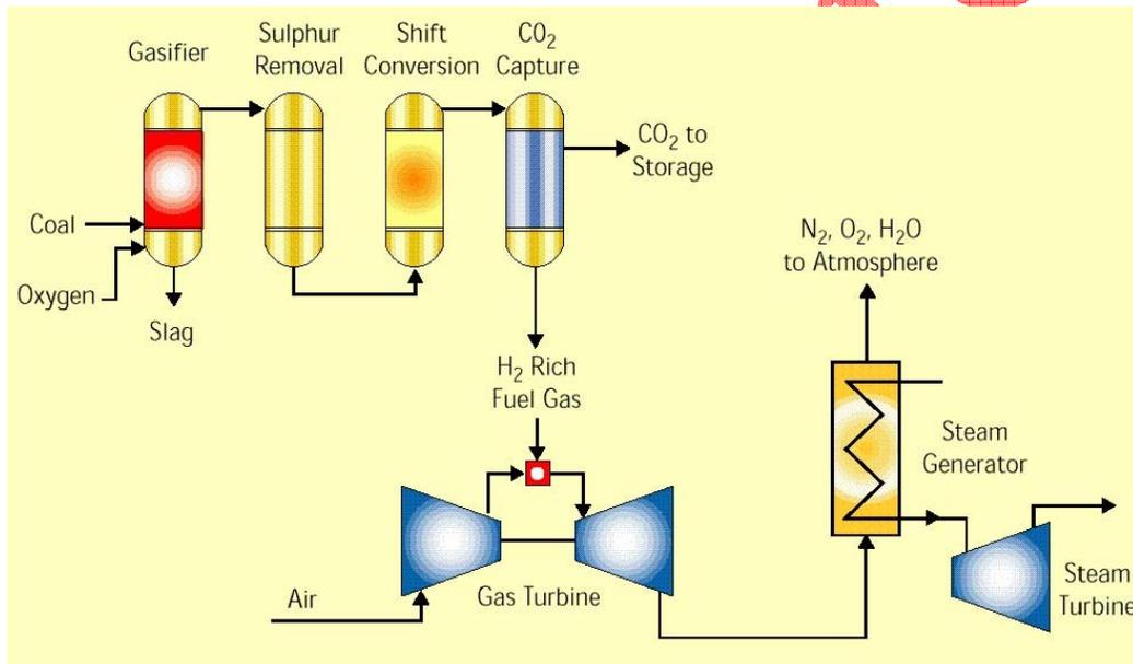
**Figure 2. Coal-fired IGCC with pre-combustion capture of CO<sub>2</sub> (courtesy of the IEA Greenhouse Gas R&D Programme)**
