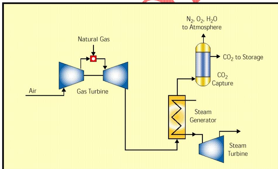
*Figure 1. Gas turbine combined cycle with post-combustion capture of CO<sub>2</sub> (courtesy of the IEA Greenhouse Gas R&D Programme).*
